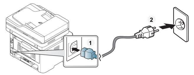
For M267xN and M287xND, also press the (Power/Wakeup) button to turn the machine on.
